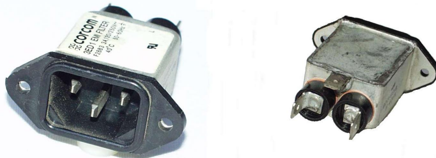
Figure 43 Chassis Power Connector that meets BFG Needs
