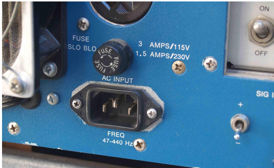
Figure 47 Power Connector that Complies with BFG Principles
