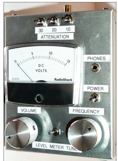
Figure 5 — Noise receiver front view.
