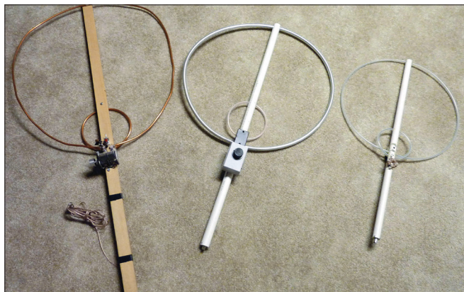
Figure 2 — Tracking loop antennas. Left to right: 24-inch copper loop, 20-inch aluminum loop, 16-inch #22 AWG wire loop with plastic tubing.
