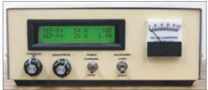
Figure 3 — Front panel of power meter. The LCD shows the peak envelope power (PEP), the average envelope power (AEP) and the SWR. The two knobs control the contrast and back lighting of the LCD. One toggle switch determines whether forward or load powers are displayed. A second switch sets the averaging time for the AEP calculation. The meter shows the SWR and is used for tuning purposes.
