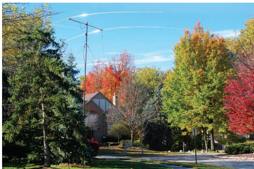
The home station of Pete Gladysz, K8PGJ, was upgraded to a four-station low power M/M for the W1AW/8 Michigan operation. This homebrewed two-element portable beam for 20 meters supplemented Pete’s two two-element SteppiRs, and verticals on 20, 17, and 2 meters, all of which are permanent antennas. [Pete Gladysz, K8PGJ, photo]
